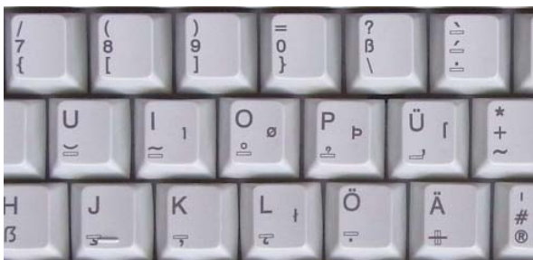
Fig. 1: Detail of a German standard keyboard according to DIN 2137-1:2012-06, showing several instances of the ISO/IEC 9995-10 base mark for diacritical marks to be entered by the dead key method.
